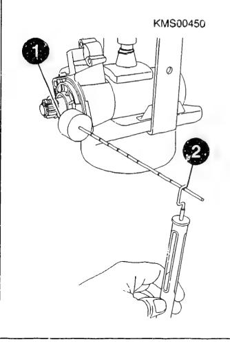
Checking clutch overrunning torque
